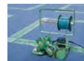
For large contract projects it is worth using an automatic welding machine.
