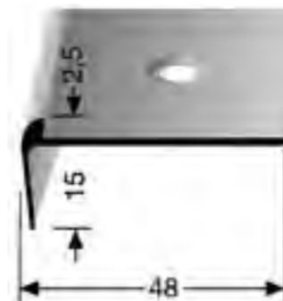
29333 – for DLW Linoleum, DLW Vinyl and DLW Luxury Vinyl 2.0 mm to 2.5 mm thick.
